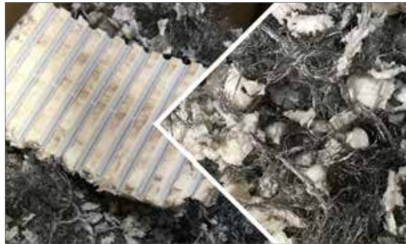
V-belts (thermoplastic with steel reinforcement)
